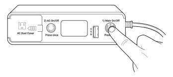
Once the Main On/Off button is pressed for 3 seconds and released, the screen will display these icons:
