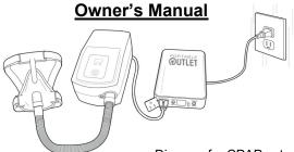
Diagram for CPAP set-up at home. Also works as a stand-alone battery.
